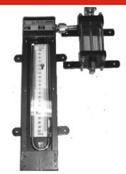
'TELELIN' High Accuracy, fully enclosed, Industrial Grade High Vacuum, Mercury Filled by evacuation, Absolute U-Tube Manometer, wall mounting type. Manometer will have 304 S.S. wetted parts. Model No. HVM-450 + SP-45 (i.e., catch-pot). It will measure vacuum in its' last stages i.e. from 560 to 760 Hg. in steps of 1 mm Hg
